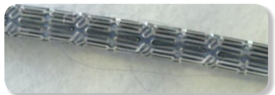
Cotton Towel Fiber found trapped on Stent strut.
