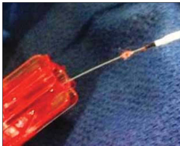
Figure 1. Cotton gauze fibers adhered to a guidewire between the tip of a balloon catheter and the Tuohy-Borst valve.
